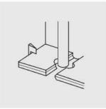
Lay the panels in places with pipes so that In rows with double pipes, follow the the pipe runs along the joint line between the panels. Choose a drill bit with a pipe diameter plus 16 mm. After snapping the panels on the short side, drill a hole in the middle of the panel joint. Now the panels are ready to be installed.
