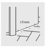
If the door frame is installed after the flooring, ensure a 1 mm gap between the bottom of the frame and the floor surface.
