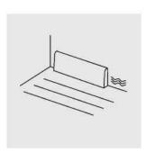
Install baseboards along the wall without attaching them directly to the floor. This will allow the floor to expand and contract. Do not fill expansion gaps with silicone.
