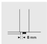
At thresholds and doorways, undercut the doorframe by laying the panel with the underside up and placing it against the doorframe. Use a multi-tool or hand saw to cut the frame at the correct height, keeping the expansion gap at 8 mm. Remove waste and vacuum the surface. Install the panel by sliding the short side close to the undercut frame and the long side toward the already installed panel. Use a tightening and/or tapping tool to ensure a solid connection.
