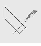
When installing, mix panels from If you need to shorten the panel different packages to avoid with a crosswise, straight stacking too many boards of cut, Pacific Vinyl Floors Herringbone UniZip should be cut with the pattern side facing up, using a special vinyl panel cutter. To cut the panel, draw a straight line along which the cut will occur. Using a knife, cut the surface along this line. There is never a need to cut the panel completely. (Hint: integrated substrate should also
