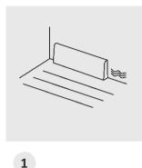
Mount the skirting boards against the wall, not attaching them directly to the floor. This will allow the floor to expand and contract. Do not fill expansion joints with silicone.
