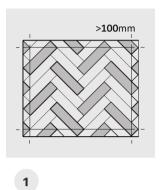
Before installation, measure the length and width of the room to correctly plan the layout of the floor rows. Make sure the last row is not narrower than 100 mm by moving the center line if necessary.
