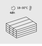
Store Pacific Vinyl Floors panels on a flat surface, in even piles, away from moisture and extreme temperatures (35°C). Acclimatize them for 48 hours at 18-30°C before installation at the installation site. Maintain this temperature before, during and for 24 hours after assembly. Carry out installation at an ambient temperature of 18-30°C and substrate temperature above 15°C.
