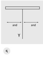
The herringbone pattern usually starts from the center line. Use a straight patch or string to mark the "Y" line.
