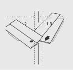
Place the first stave at a 45° angle. Draw additional lines "L" and "R" running parallel to the "Y" line to determine the position of the corners of the stave. Then draw an "X" line as shown.
