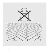
Pacific Vinyl Floors should not be blocked. Heavy objects such as kitchens and permanent furniture structures, should be installed before laying the floor. Heatemitting objects, such as stoves, must be placed on protective panels, and the panels must be around them. arranged maintaining adequate expansion gaps.
